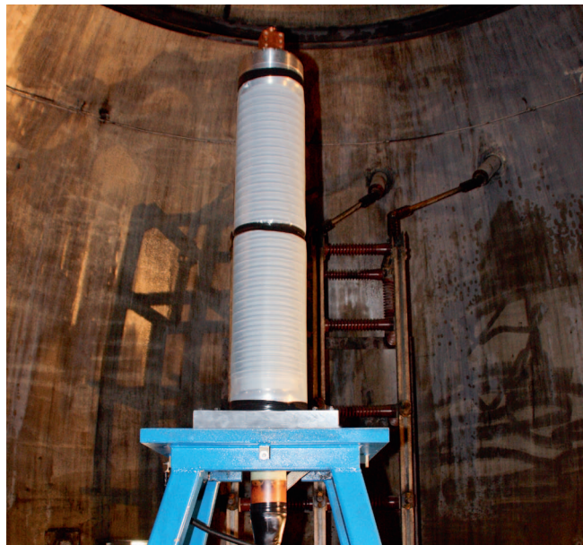
Explosion resistant termination during the test in a PEHLA Laboratory.
